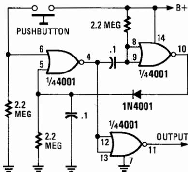
FIG. 12—SIMPLE TEST CIRCUIT produces a single bounce-free output each time you push the switch.
