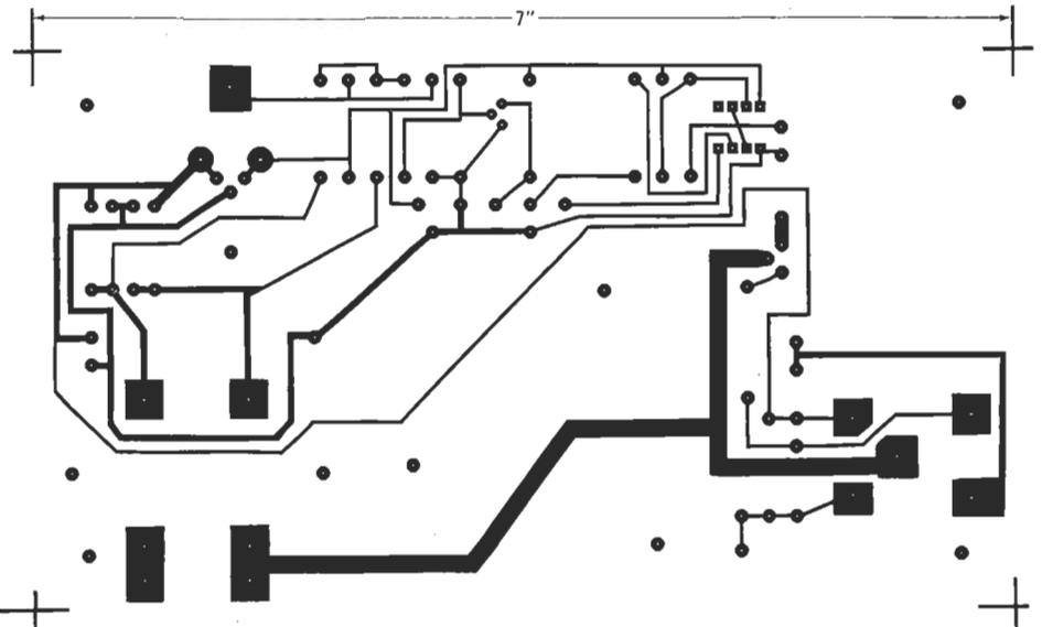
FIG. 7—THE POWER SUPPLY CIRCUIT BOARD is single-sided. Again, be sure to note the dimension across the top as this board is not drawn actual size.
