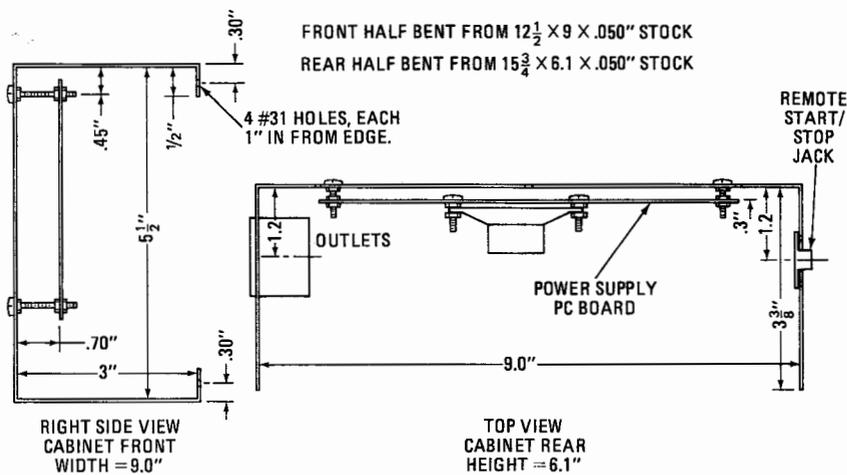
FIG. 11—CASE BENDING INSTRUCTIONS for the builder who wants to make his own case. The detail at the right shows how the speaker is positioned and mounted inside the case.
