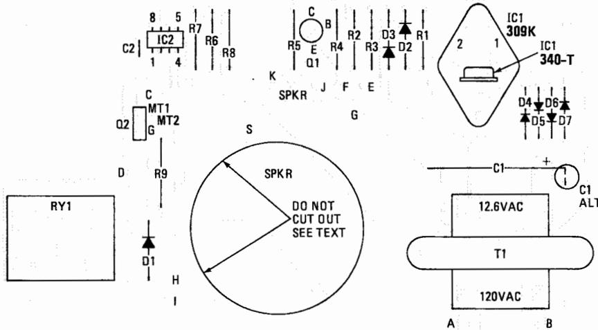
**FIG. 9—PARTS PLACEMENT ON THE POWER-SUPPLY BOARD. Note that the speaker and audio circuit components are also placed on this board.**
